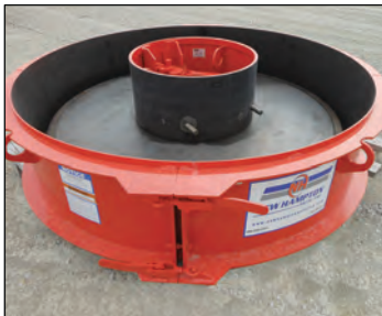
Slab Top Form
