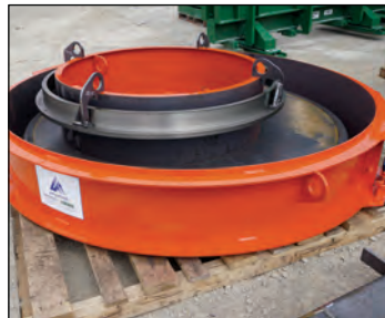
Transition Slab Form
