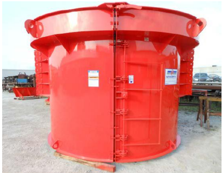
Manhole Base Form
